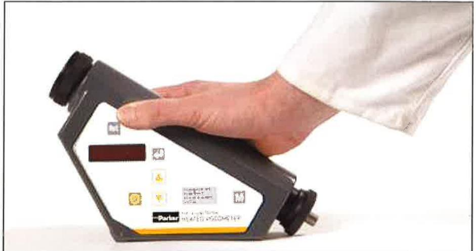
Viscosity is regarded as an oil's most important characteristic. It is the viscosity that shows the oil's resistance to flow and the strength of the oil film between surfaces. Viscosity can increase or decrease as a result of problems such as contamination, fuel dilution and shear thinning. Measurement of viscosity is extremely important for hydraulic oils, diesel engine oils, gears and fuel oils.
